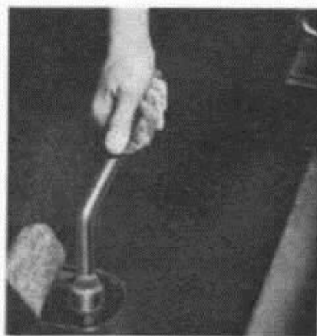
Fig. 9. Lowering the spare wheel.
