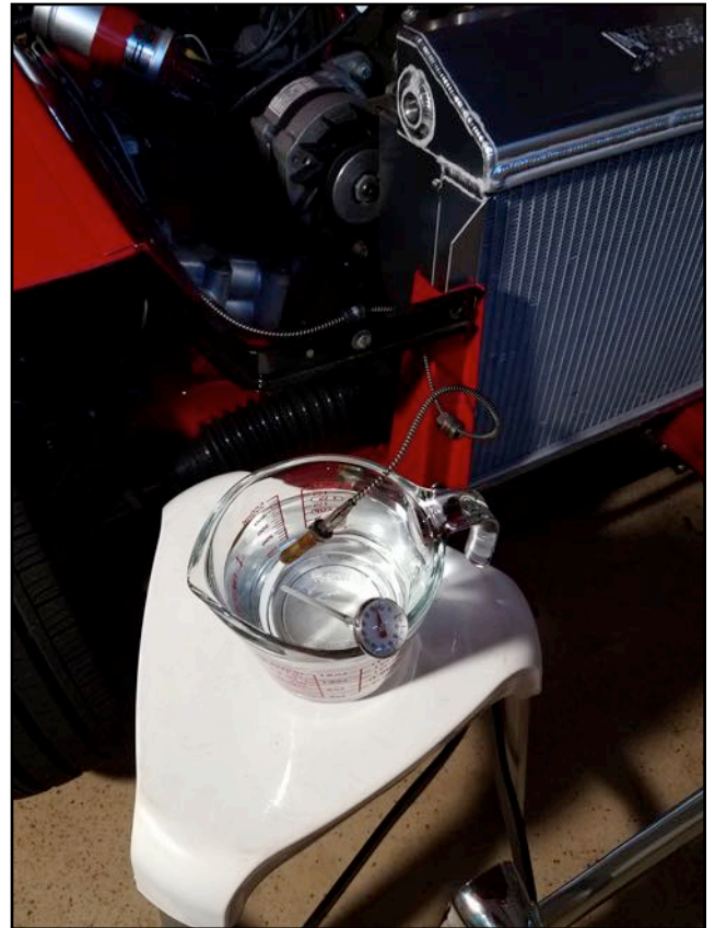
Scientific testing process (temperature gauge-thermometer calibration)
