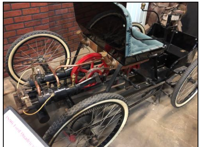
1896 Ford Quadricycle. No brakes! Driver pushes a foot onto the front tire.
