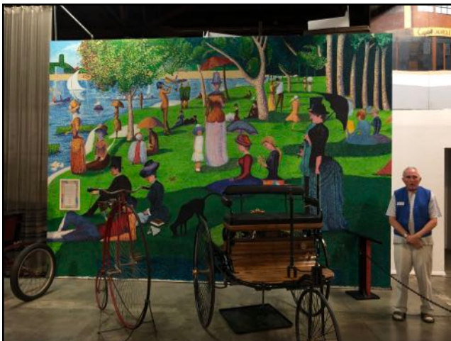
1886 Benz and bicycles. Benz brake was a belt pulled against a drum on the axle.
