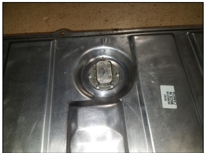
Removing the old sending unit
