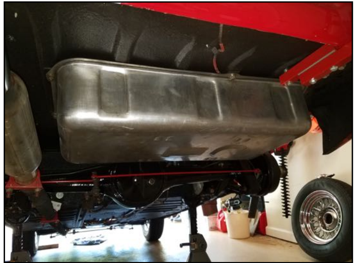
Removing the fuel tank
