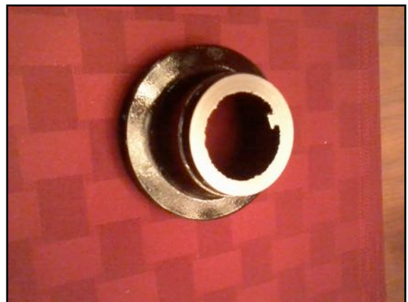
What's left of this pulley is what happened after too much time in the lathe
