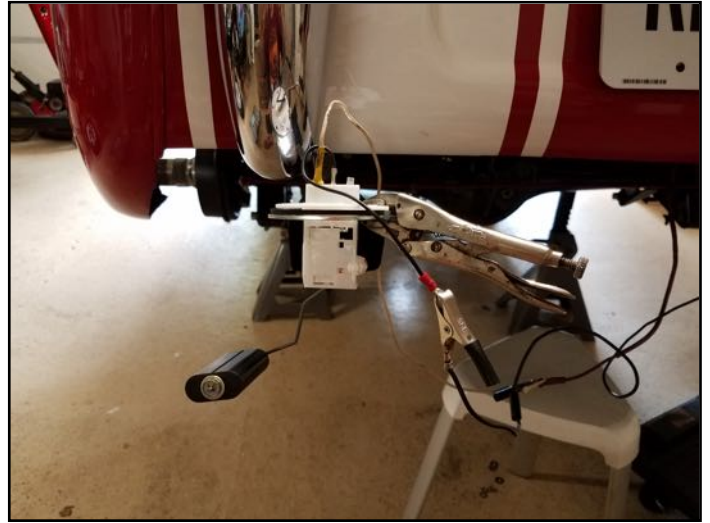
Testing the new sending unit
