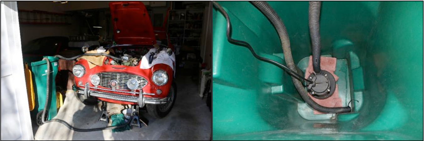
Sump pump rig for flushing out engine block waterways
