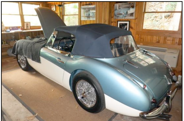
Top layer folded back to show the second added layer. Note the part touching the fender is white making it easier to keep clean
