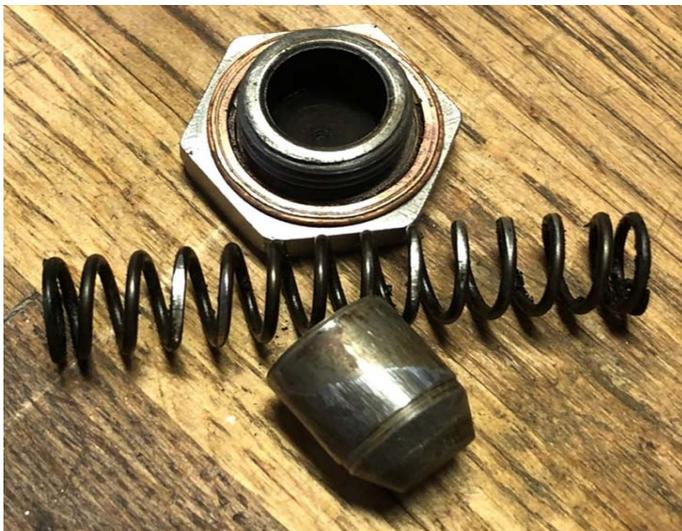
You saw the worn main bearings above. Here is a photo of the oil pressure relief valve. Note the flat shiny spots that have worn (from vibration) on the spring; these areas of lost metal will reduce the spring's strength.
