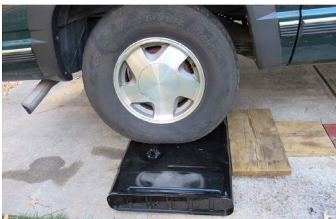
Well, that did not go as expected. The tank held up to having a truck drive over it!
