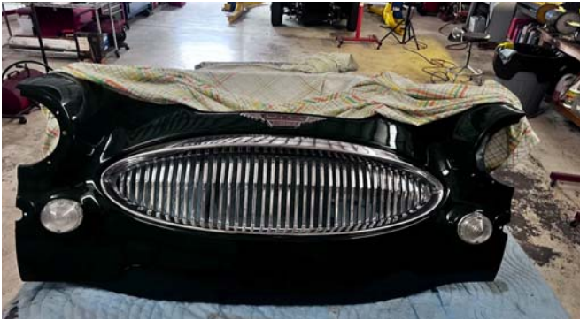
Bennet has put the grille back into the front shroud and that will be finding its way onto the chassis soon.
