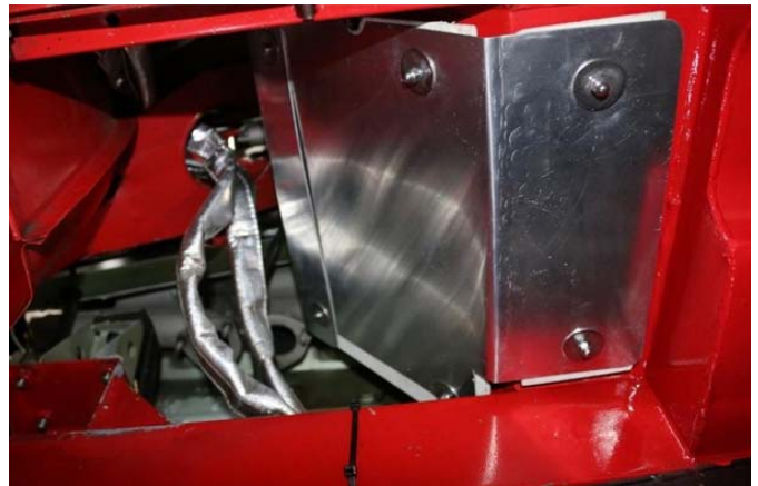
The finished product. My metal fabrication skills just went from zero experience to something slightly north of that. I'm not anywhere close to being a "panel beater", but I am quite happy with how everything came together and bolted up. The silver cloth tubes in this photo are to protect the oxygen sensor cabling from adjacent exhaust pipes' heat.
